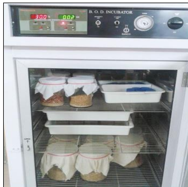
Fig 2: BOD incubator to study various levels of temperature & RH under laboratory condition
