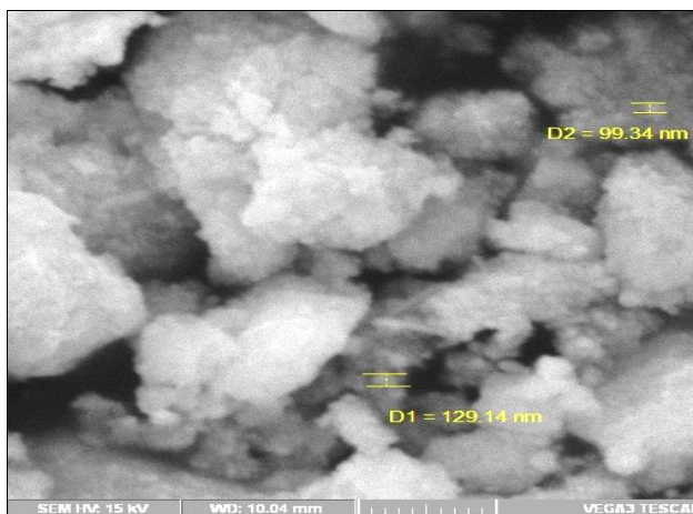
Fig 8: SEM image of silver nanoparticles synthesized by W. tinctoria leaves extract
