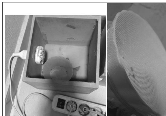
Fig 1: Plastic jars covered with fine small bores muslin introduced into the fumigant chamber of approximately 6 L with fumigant electric device
